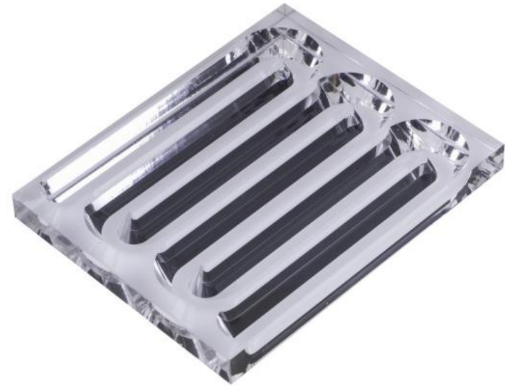
Counting Chamber Based on Bogorov Design
